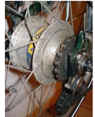
Dickes Ding: Rohloff Speedhub 500/14
